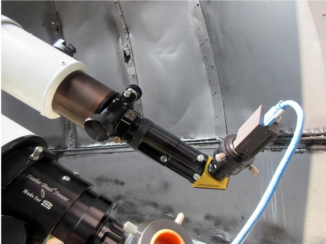
Figure 8- TMB 100 mm F/8, PST Stage 2 Mod (CCD imaging).
