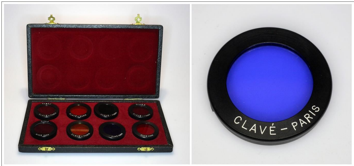
Figure 10- Clavé eyepiece colour filters (Pedro Ré's personal collection).
