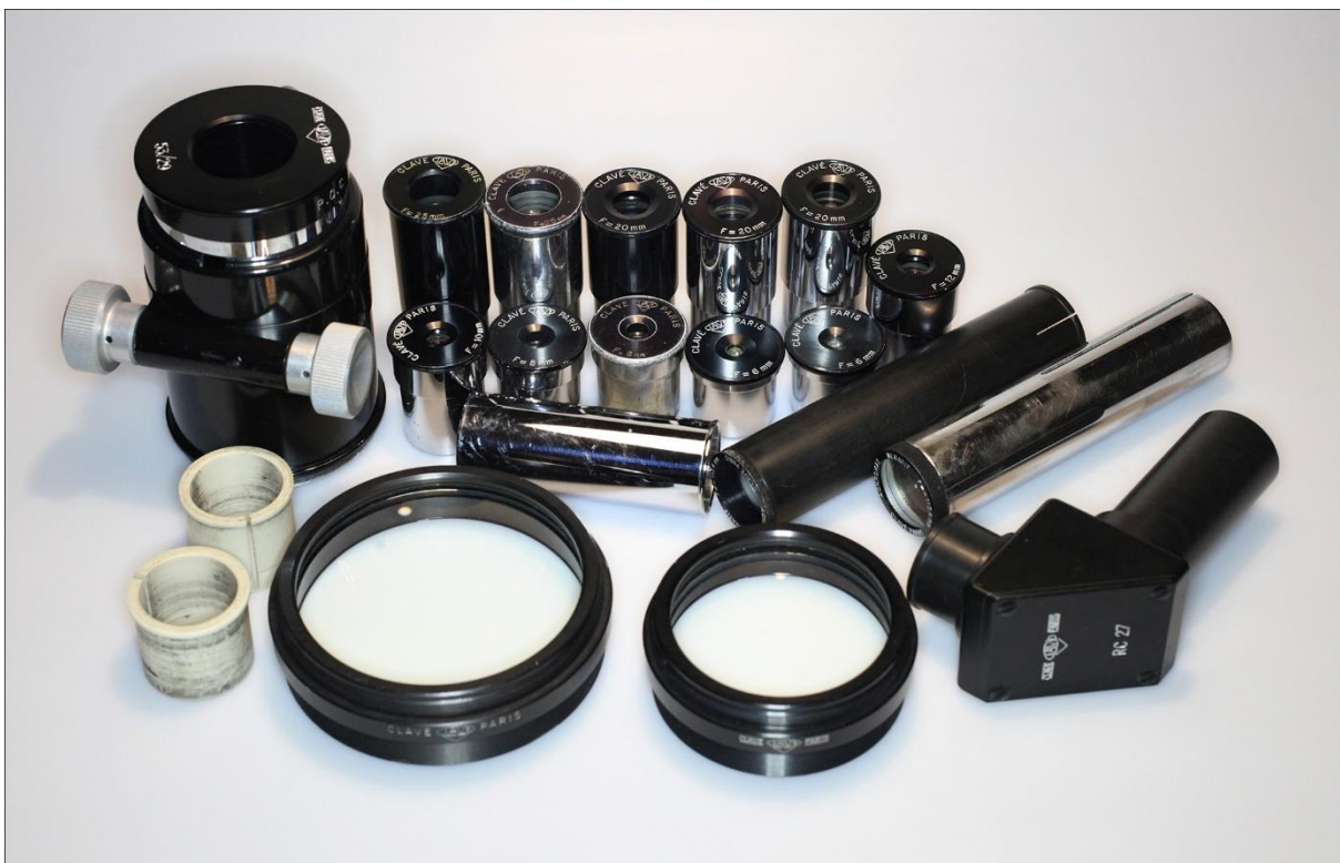
Figure 11- Clavé 27 mm eyepieces, focuser, prism, barlow lenses, objectives (Pedro Ré's personal collection).
