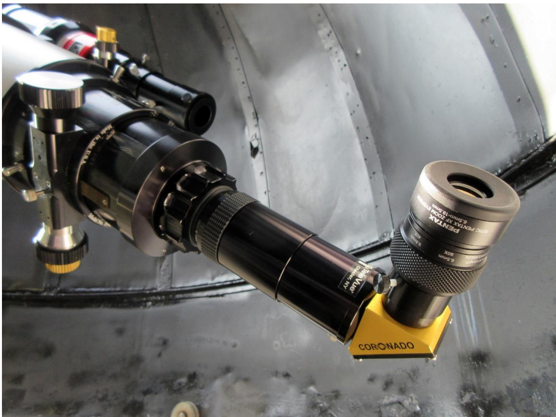
Figure 11. TEC 140 mm F/7, PST Stage 2 Mod (visual observation).
