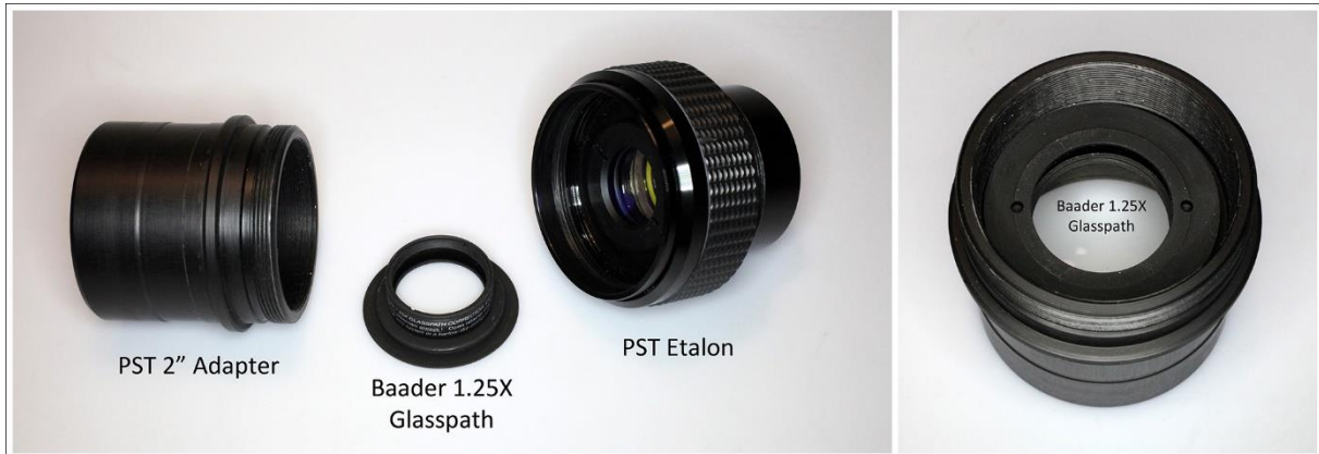
Figure 4 – PST etalon + Baader 1.25X Glasspath.
