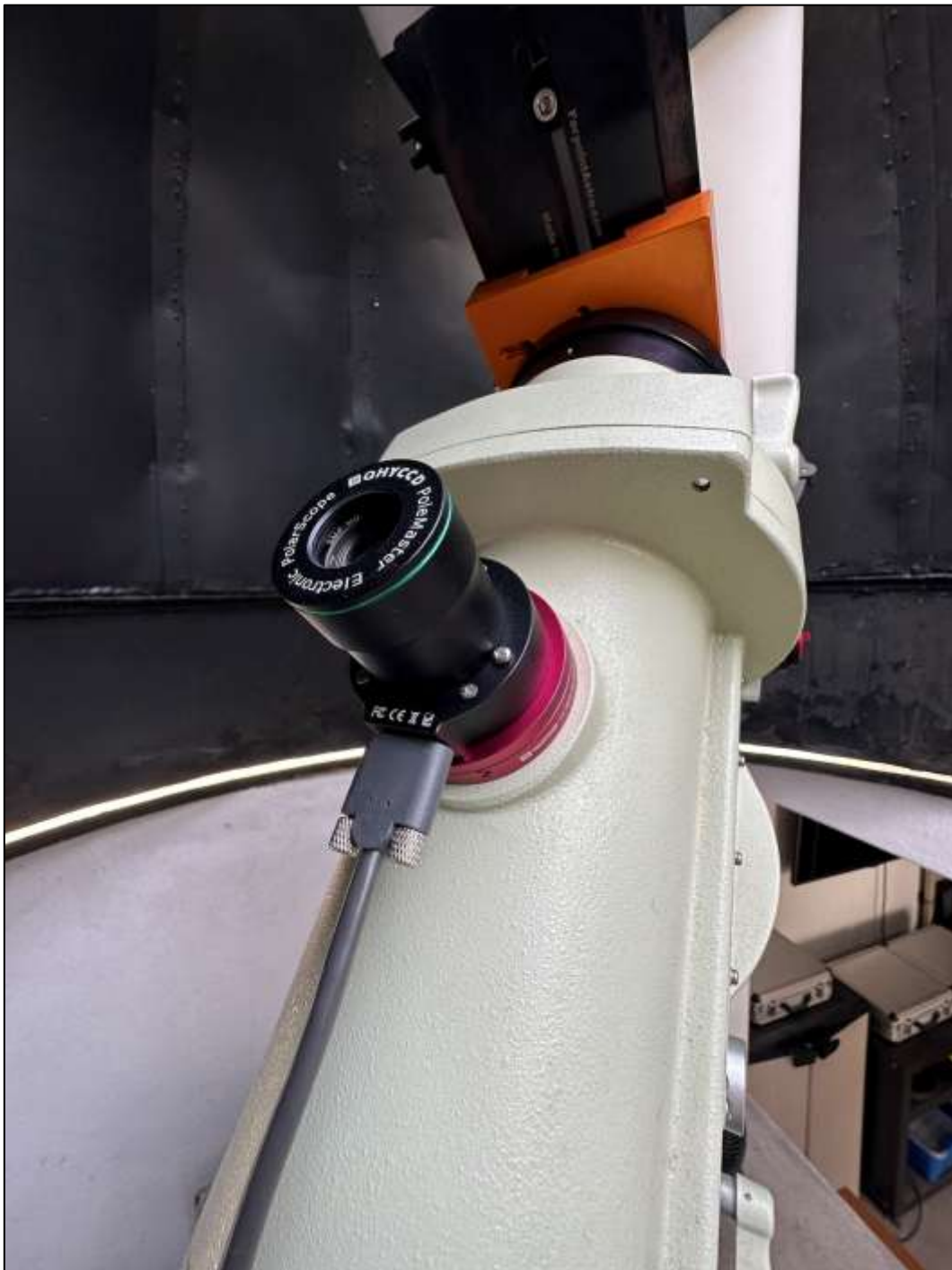
Figure 2- Polemaster installed on a Takahashi EM400 mount.
