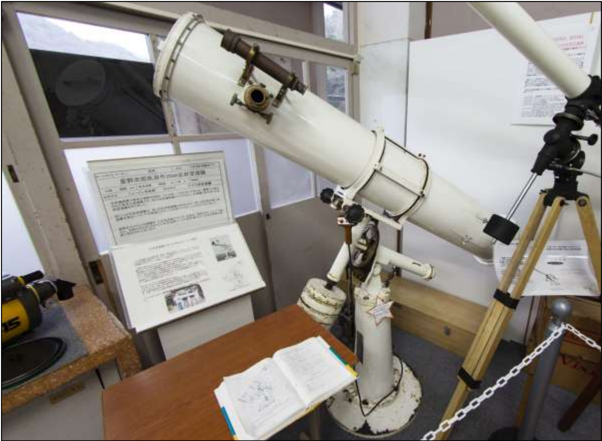
Figure 13 – 20 cm reflector made by “Jiro Hoshino” one of the pioneers of Japanese amateur telescope making and astrophotography.
