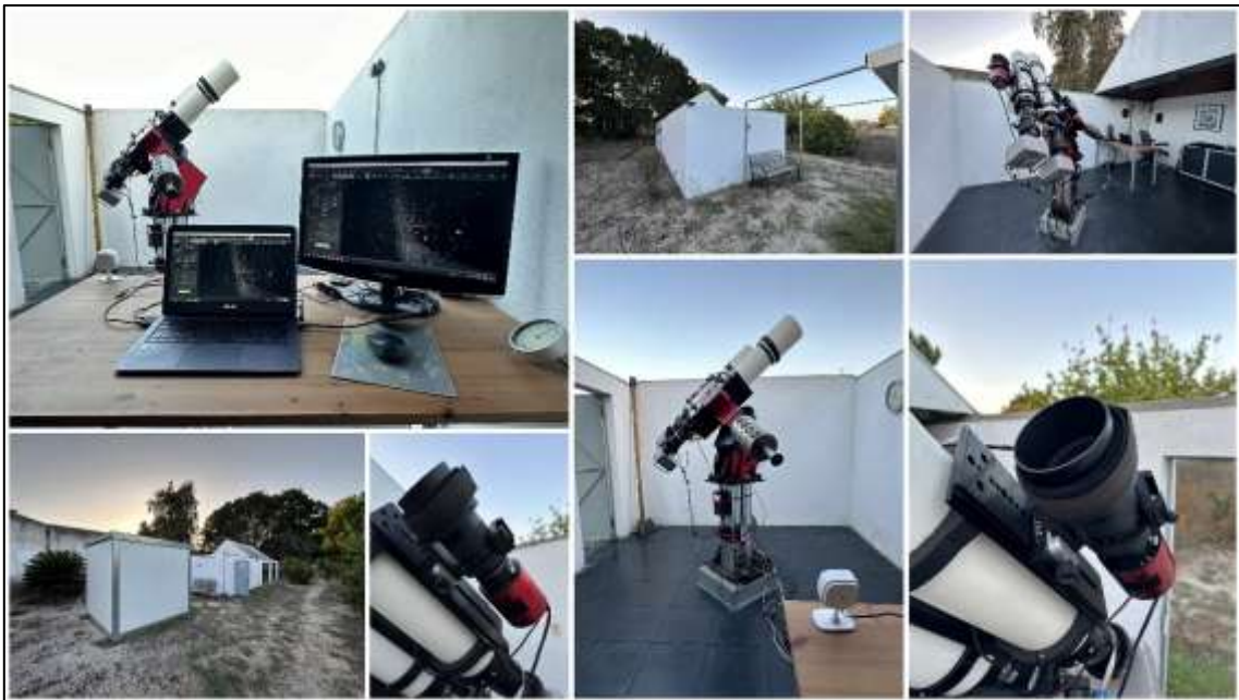
Figure 13- Imaging setup. First light with the ZWO ASI2600MM & Samyang 135 mm f/2 (20231004).
